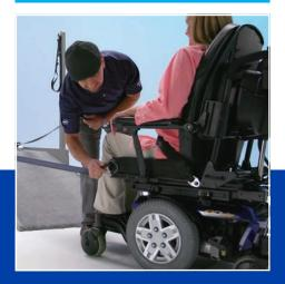
The operator releases the INQLINE belts and attaches J-hooks to the wheelchair frame to secure the mobility device.
