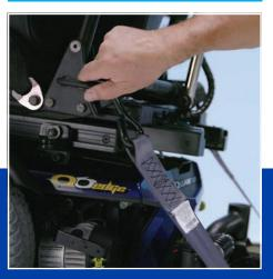
Once safely inside, the operator attaches the rear tie-downs and applies a 'final squeeze' via the wall control unit.
